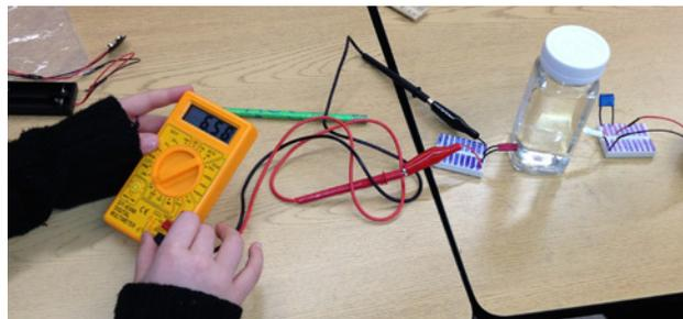
Figure 2. Students record the voltage of their photoresistor circuit in response to the amount of light from an LED circuit as the LED is moved away. Then, a solution, representing one of the eight environments, is placed in the path to determine the relative amount of light that penetrates the solution.
