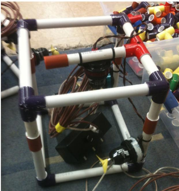
Figure 3. Students design a frame that supports three thrusters that are wired to a control box. Buoyancy (not shown) is then added to the frame before testing in a 300-gallon tank (a plastic "horse trough" that is roughly 2.5-feet wide, 6-feet long, and 2-feet high). These initial tests usually spur modification to the ROV and further testing.
