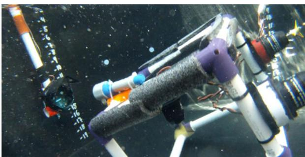
Figure 4. An ROV with flashlight attached to the top of the frame drives near the photoresistor to "download data." Portions of a secret code are displayed with a score that depends on the amount of light recorded by the photoresistor in 30 seconds.
