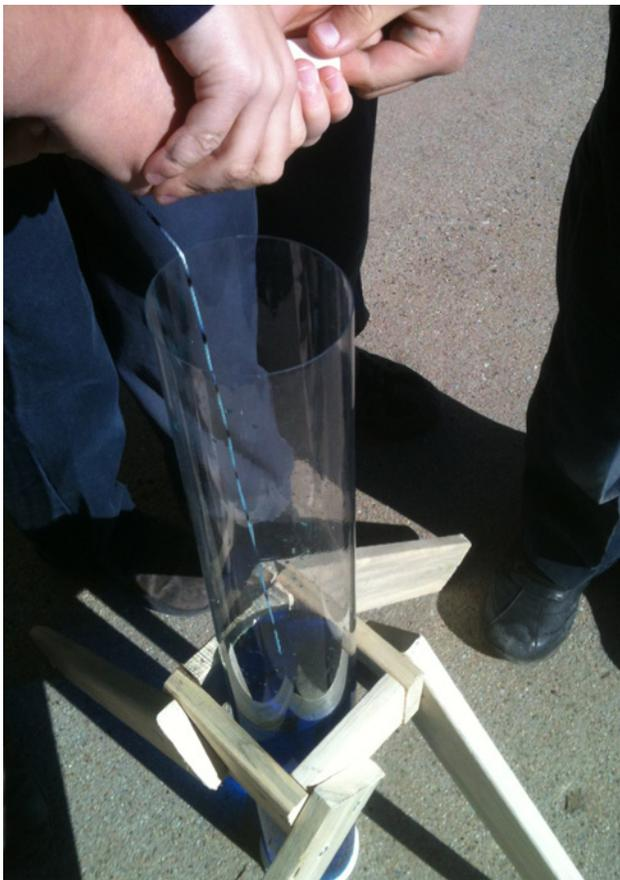
Figure 1. Students raise and lower a Secchi disk to determine the turbidity of the solution, which represents one of eight environments from rivers to open ocean. Solutions are made of colored dyes and fine-grained sediment.
